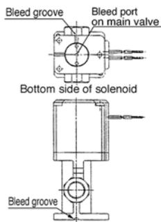
2. Take proper measures to prevent dust or foreign matter from entering through unused ports. The grommet portion contains a breather hole for the core. Take proper measures to prevent dust or foreign matter from accumulating in this area.
