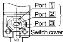
Port positions for manifold solenoid valve body.
