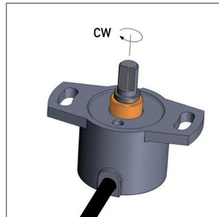
When the shaft marking points toward the cable outlet, the sensor is located in the electrical center position.
