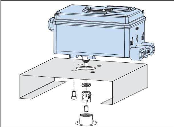
**Attention:** The feedback shaft **9** of the SRI has no mechanical stop, therefore may spin 360 degrees. The permissible rotation angle range is between +50 and -50 degrees around the arrow at the housing concerning the flat area of the feedback shaft (also see detail page 13 bottom). Since a rotary actuator has a rotary angle of about 90 degrees the mounting as described in the following must be carried out very precisely.
