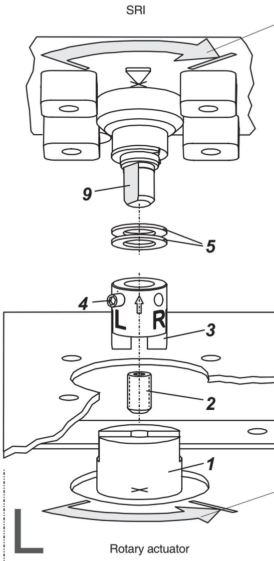
Figure 27: Mounting if actuator is rotating to the left
