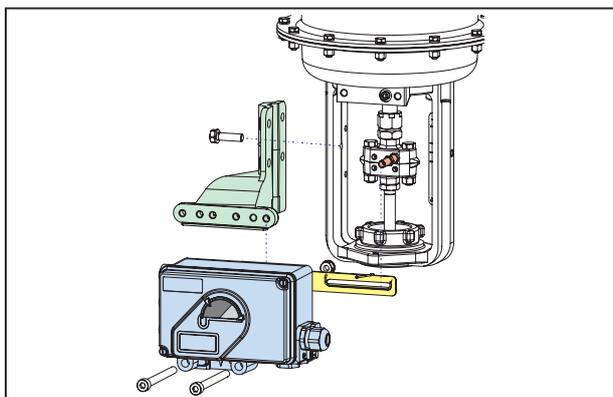
Attachment of the positioner to the actuator is made to the left using the mounting bracket and feedback lever for a NAMUR mount. Use:
