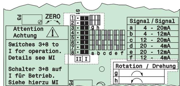
L: left-hand rotating feedback shaft      switch 1+2 on "I"
