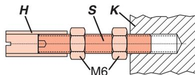
It consists of a stud **S**, which is screwed into the coupling piece **K** (with 3 mm Allen key) and locked with a lock nut M6. The threaded sleeve **H** is screwed onto it and locked with a lock nut M6. Make sure that the bolt is adjusted to the right length!
