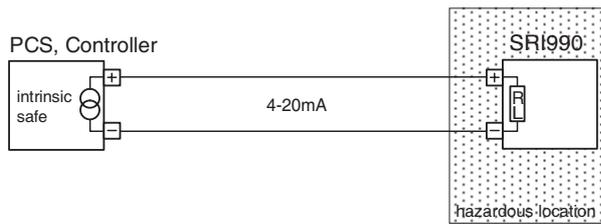
Controller / process control system-output not intrinsically safe:
