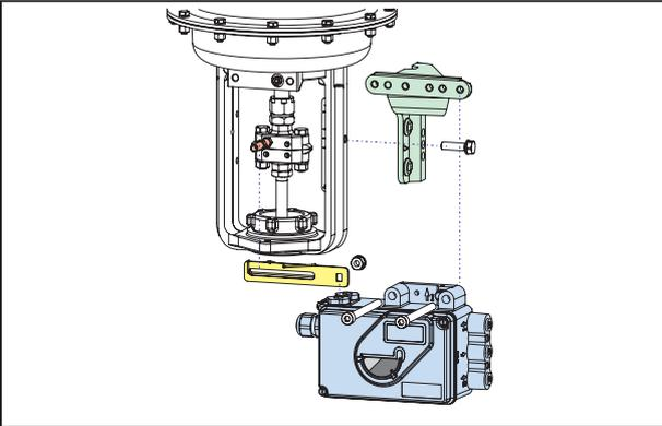
Attachment of the positioner to the actuator is made to the right using the mounting bracket and feedback lever for a NAMUR mount. Use: attachment kit EBZG -H for a cast yoke, or attachment kit EBZG -K for a pillar yoke.
