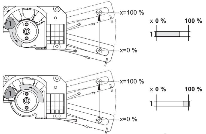
**Setting limit switch trigger points**
