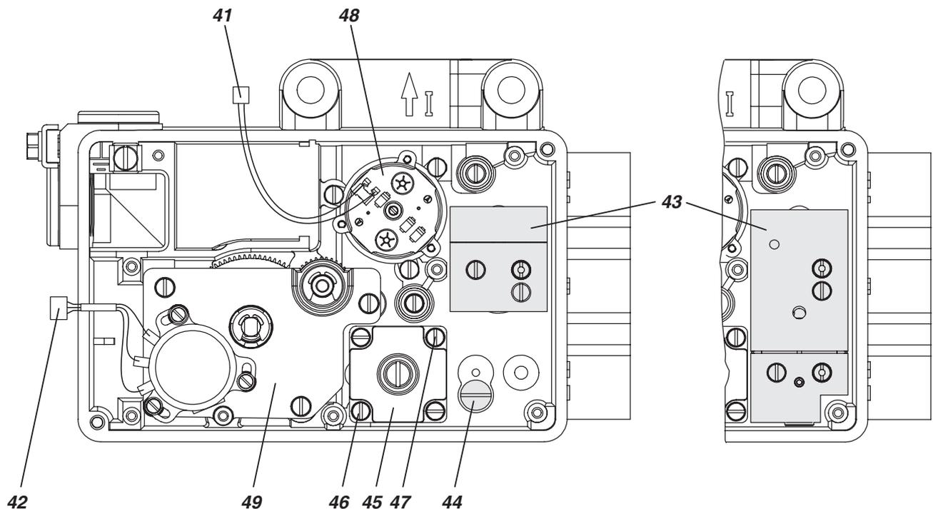
1) The base plate consists of a manifold and air ducts. O-rings are required to guarantee sealing of the mounted elements.
